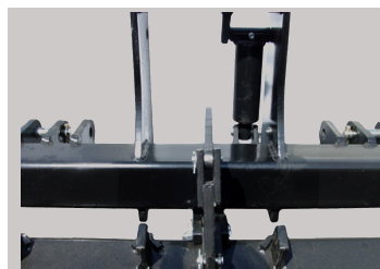
New cylinder and heavy, long lasting linkage brackets
